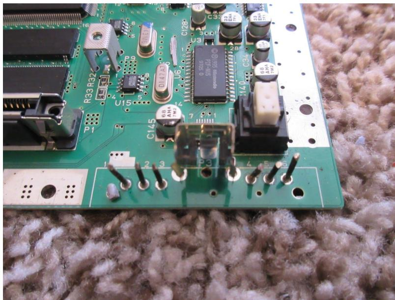
After that, snip off the remainder of the prongs, and bend that metal thing in the middle back and forth until it snaps off.
