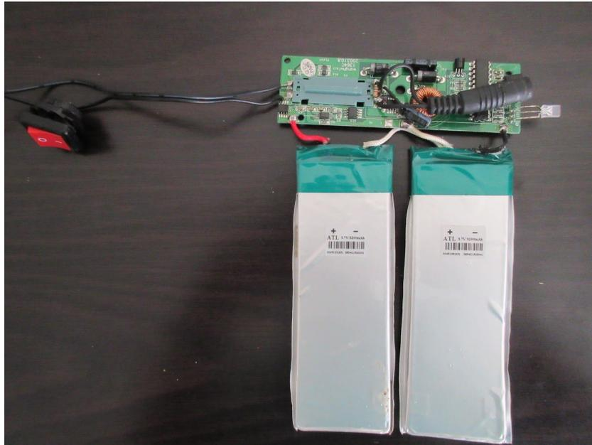
Generally, people use two 3.7v cells wired to a protection circuit to prevent overcharging and over discharging. In the picture above, the two cells and pcb are clearly seen as well as a power switch on the +7.4v line.
